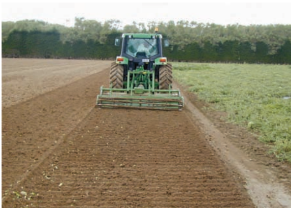
Figure 16.5. Powered tillage tools used with horticultural crops: rotary tiller (left), and spader (right).
