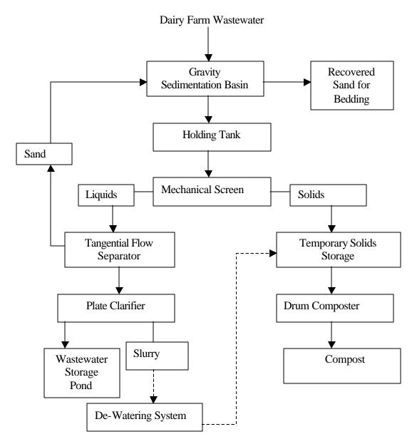
Figure 3-1. Flow diagram of the nutrient removal and composting system at Gore's Dairy, Zephyrhills, Florida. (Nordstedt & Sowerby, 2000)
