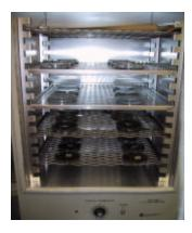
Figure 3-3. Incubator used for germination tests.
